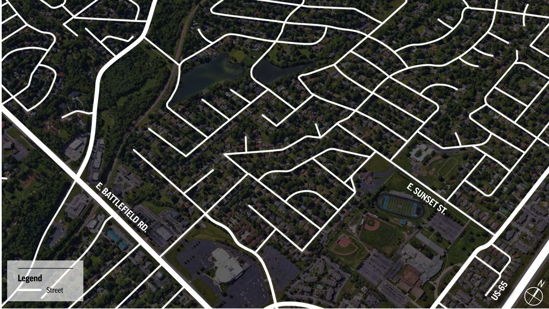
Suburb Block Pattern Block Size: approx. 4 acres through 16 acres Block Dimensions: approx. 325' x 565' through 1,220' x 575'
