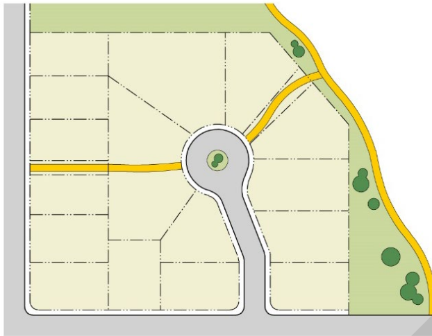
Figure 3-4 Walkways and Bicycle Routes. Where streets will not connect or where larger blocks are platted, connections for pedestrians or bikes may be required through blocks or at the ends of disconnected streets. (3.01.B.3).
