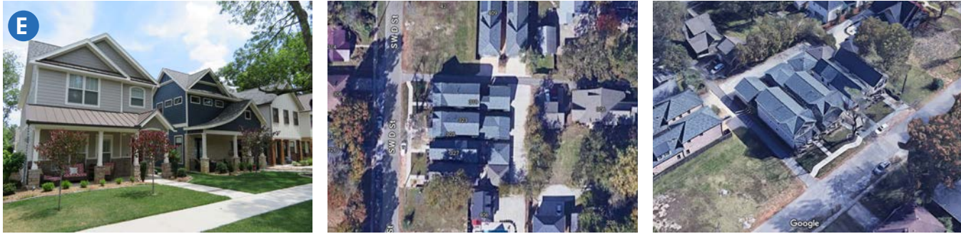
Housing Type: Small Lot Single Family Total Housing Units: 4 | Area: 0.45 acres | Density: 8.8 units per acre | Access: Side Lot Access
